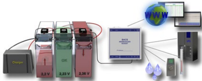
Picture: The BACS WEBMANAGER controls the battery voltage of batteries 1 and 3
